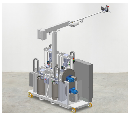
Design example of NODOPOX wind with refilling (4-drum system) and pneumatic unwind and re-wind unit for power and air connection cables
