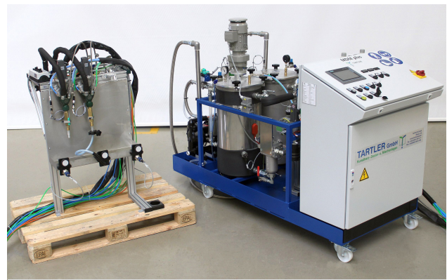
MDM plus from TARTLER for filament winding: The custom-designed system features two mixing heads for filling impregnation baths. They are controlled via level sensors.
