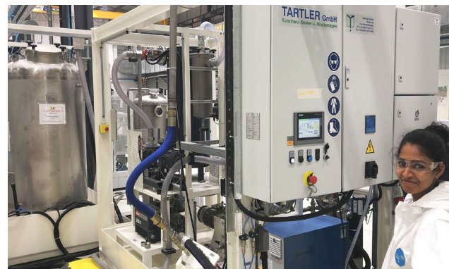
The T-EVAC from TARTLER has a Siemens PLC (7-inch HMI screen) as standard, is designed for the conditioning of epoxy and polyurethane resins and achieves degassing capacities of up to 1,000 l/h.
