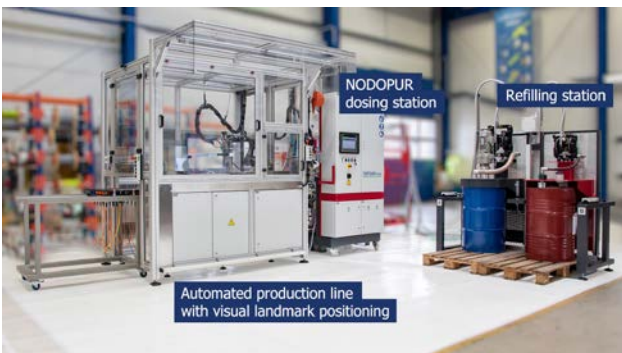
The power units of the encapsulation station: A NODOPUR dosing and mixing system, a closed cell with robot-guided mixing and application head, and a refill station.
