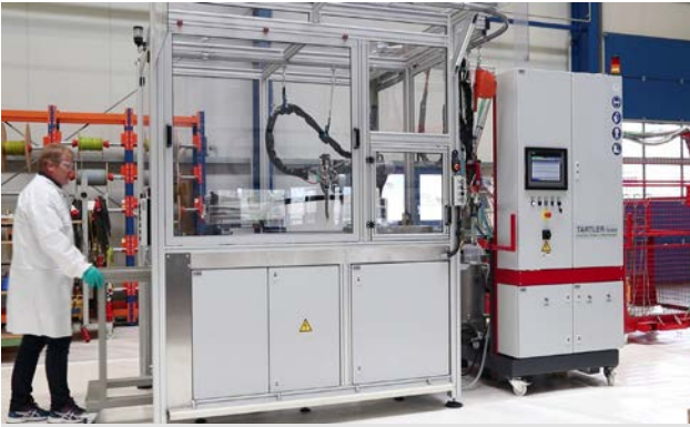
The robotic cell of the encapsulation station has a pneumatic gate for moving a workpiece carrier in and out, sensors for sensing distances and positions, and windows that allow easy access to the system.
