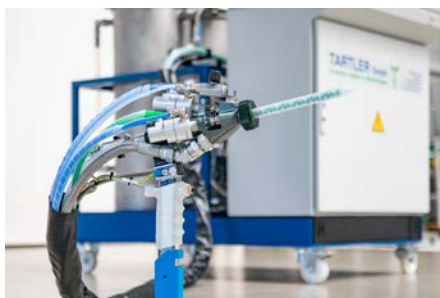
The MDM plus is equipped with the LC5/3 mixing head.
