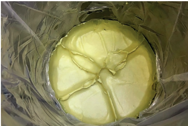
Even with a carefully emptied drum, up to 14 kg of resin residues remain in the liner. They can be processed with the TAVA 200 F from TARTLER and fed back into the rotor blade production process.
