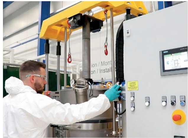
The TARTLER TAVA 200 F degassing station can be integrated directly into the filling and decanting processes of synthetic resin processing.
