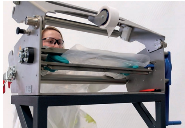
In addition to its TAVA 200 F degassing station, TARTLER offers a mobile press-out unit with which the last residues of resin can be pressed out of the inliner and collected in a drum.
