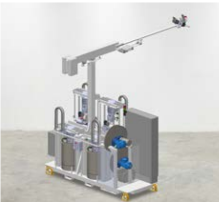
Design example of NODOPOX wind with refilling (4-drum system) and pneumatic unwind units for power and air connection cables
