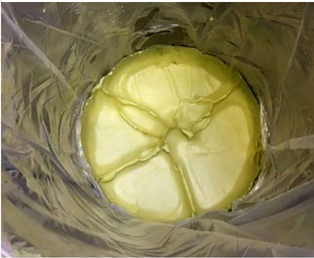
Even when drums are emptied properly, up to 14 kg of synthetic resin residues remain in the liner. The TAVA 200 F from TARTLER GROUP allows these to be processed and fed back into the rotor blade production process.
