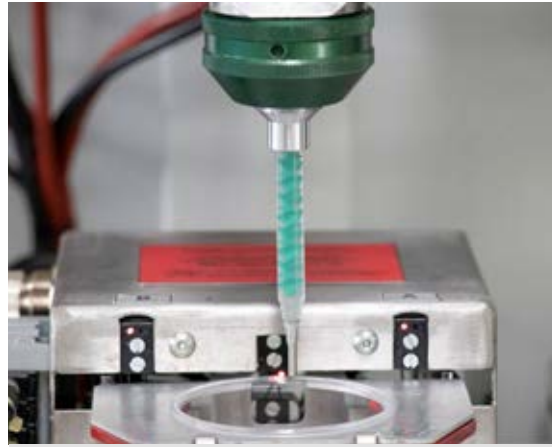
The dosing mixing head LV 2/2 from TARTLER is suitable for series processing of resins and hardeners with viscosities from 50 to 20,000 mPas in mixing ratios from 100:5 to 100:200.
