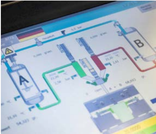
View of the four-color touch panel of the TARTLER LV2/2 dosing mixing head.
