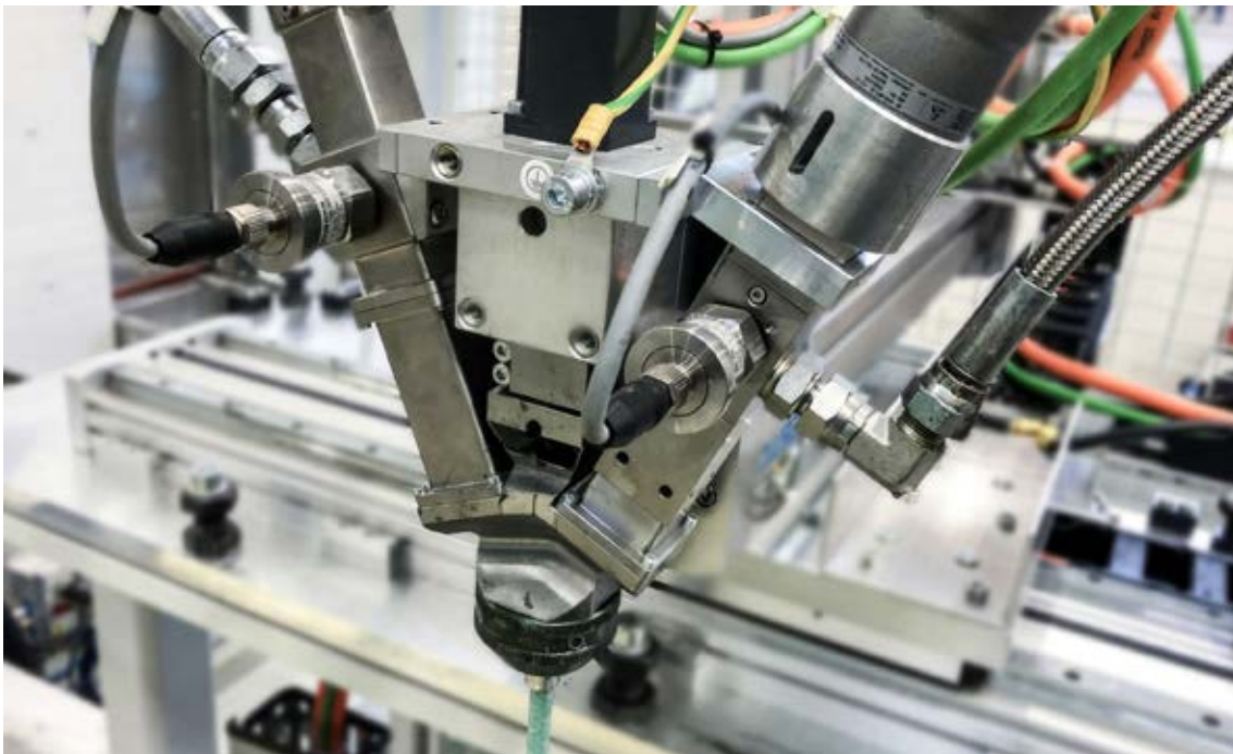
The standard version of the TARTLER LV 2/2 dosing mixing head is designed for the application of two components. However, it can also be upgraded for dosing, mixing and applying up to four components.
