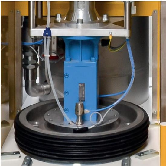
Vacuum-supported follower plate ventilation (option 2) represents the middle ground. Here, process safety increases and material loss is reduced.
