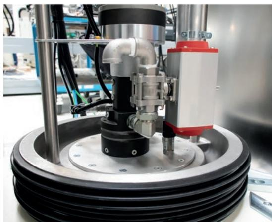
The manual drum ventilation via ball valve or similar (option 1) is problematic. It leads to material loss and splashes, and provides no guarantee for the absence of air under the follower plate.
