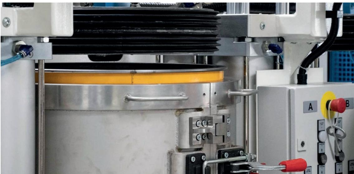
The 3rd option works with a vacuum drum (TAVA) from TARTLER, which functions like a vacuum chamber. This enables the generation of a very high vacuum (-0.97 bar) in the drum. During the drum change, no air is brought into the system, and material loss and risk of splashing are ruled out.
