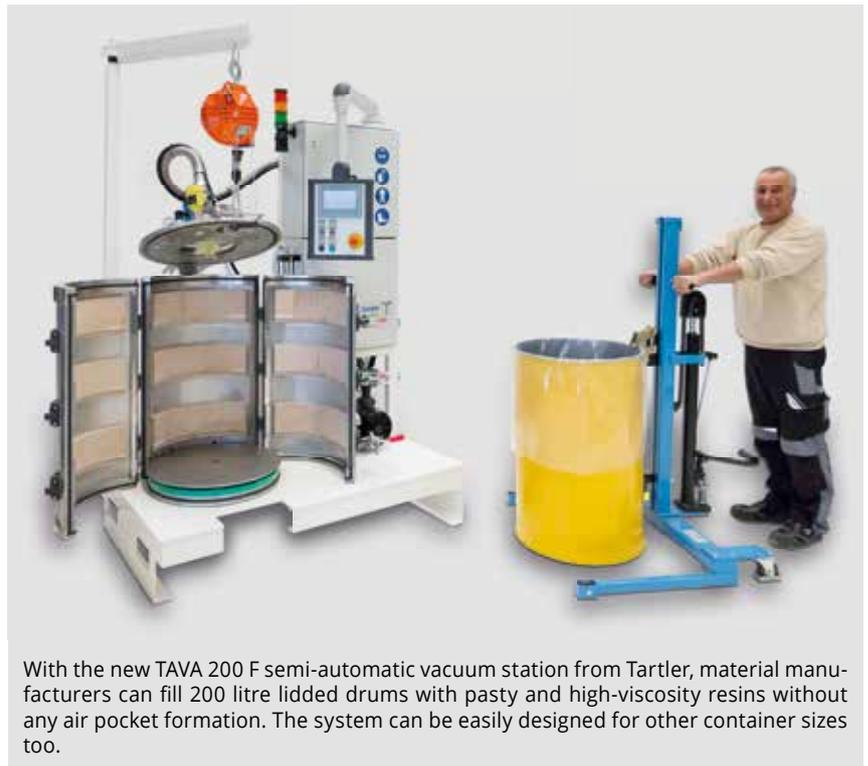
With the new TAVA 200 F semi-automatic vacuum station from Tartler, material manufacturers can fill 200 litre lidded drums with pasty and high-viscosity resins without any air pocket formation. The system can be easily designed for other container sizes too.
