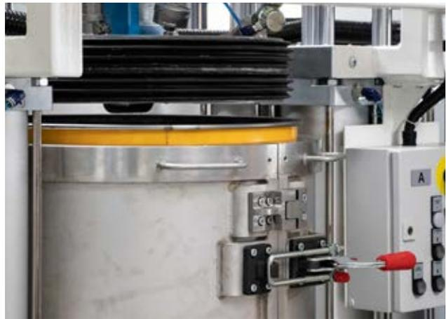
The 3rd option works with a vacuum drum (TAVA) from TARTLER, which functions like a vacuum chamber. This enables the generation of a very high vacuum (-0.97 bar) in the drum. During the drum change, no air is brought into the system, and material loss and risk of splashing are ruled out.
