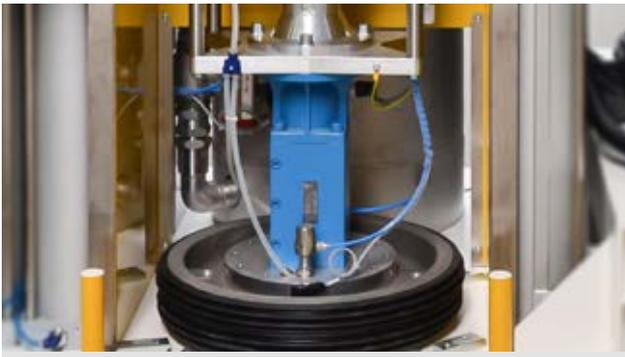
Vacuum-supported follower plate ventilation (option 2) represents the middle ground. Here, process safety increases and material loss is reduced.
