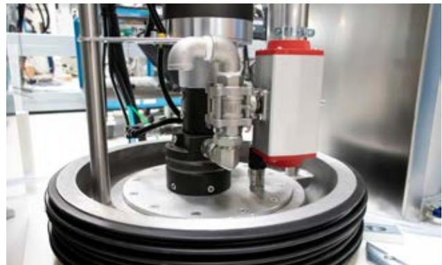
The manual drum ventilation via ball valve or similar (option 1) is problematic. It leads to material loss and splashes, and provides no guarantee for the absence of air under the follower plate.
