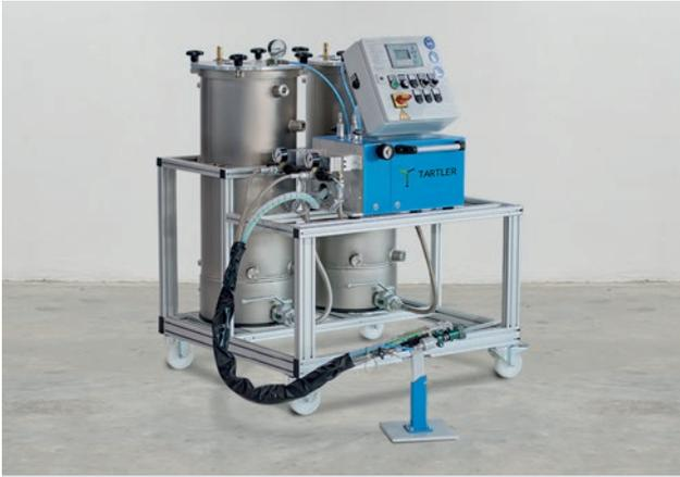
The MDM 5 from TARTLER convinces with extensive standard features and a Siemens control system with shot time pre-selection and a pot time alarm. The picture shows a variant with a chassis and large 60-litre containers.
