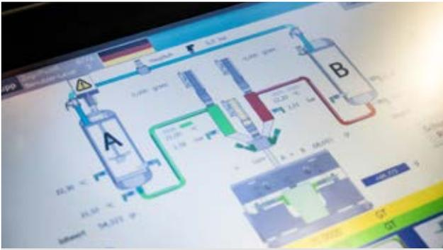
A glance at the panel of TARTLER's LV 2/2. The new dosing mixing head enables the mixing of resins and hardeners with viscosities ranging from 50 to 20,000 mPas, as well as the pinpoint and repeatable dosing of tiny shot quantities from 1.0 to 10 grams.
