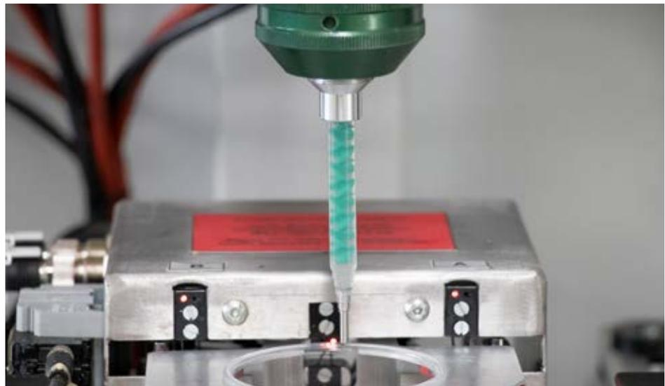
TARTLER's new dosing mixing head LV 2/2 is designed for the high-precision processing of low-viscosity components and their pinpoint application in smallest quantities. It is specially designed for demanding quality applications in electro casting and adhesive technology.
